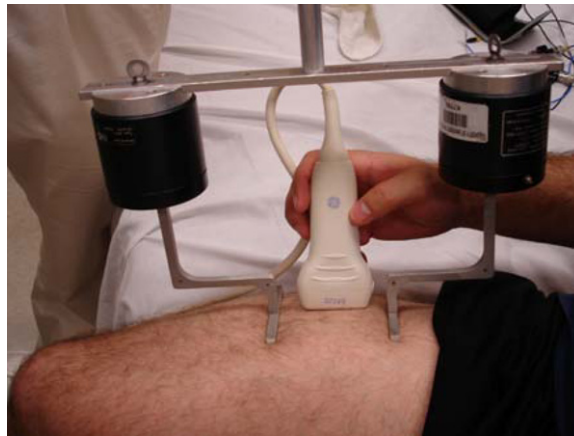
Figure 9. Representative image of the handheld mechanical source pair equipped with surface contacts and ultrasound transducer placement as used for all in vivo skeletal muscle experiments.
